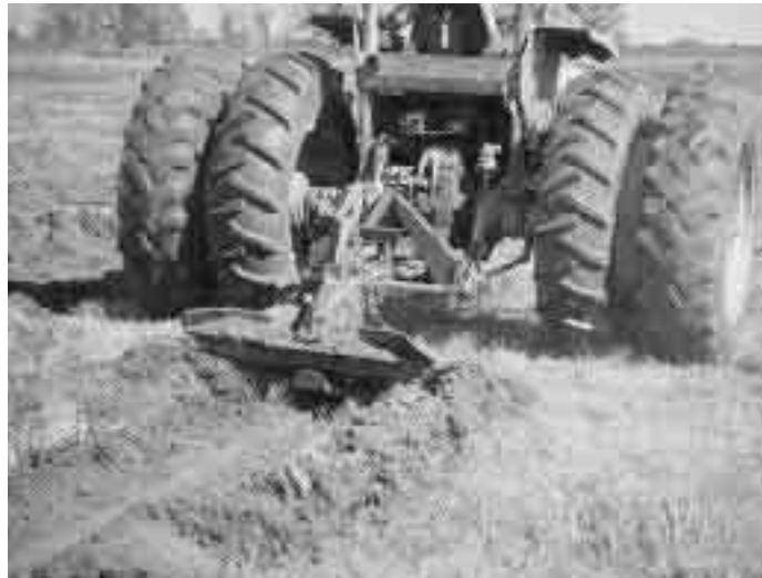
This tractor is scalping an old field site with a three-point hitch scalper.
