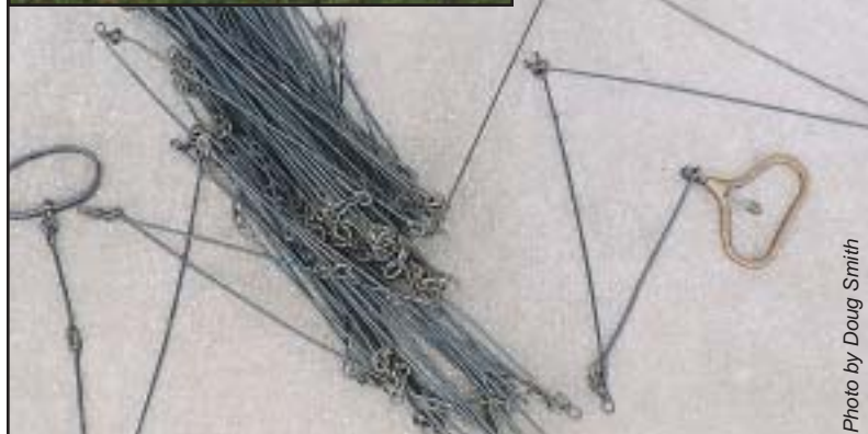
Figure 2 Top photo: Metal tape (chain) on a reel (note: may be metal or fabric). A link on one end is graduated and marked with ten divisions for increased accuracy. Bottom photo: Example of a Gunter's Chain. A surveyor's chain = 66 feet = 100 links, therefore one link = .66 feet = 7.92 inches.
